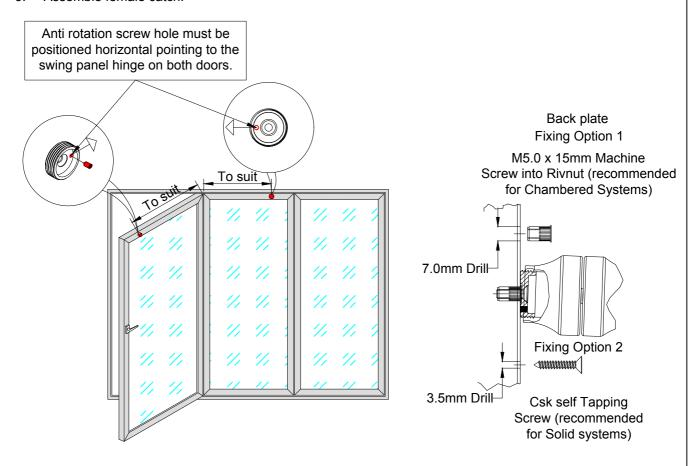
6. Connect both panel catches and mark the center position on the opposite door.
